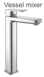
Tonic II vessel mixer with maximum 5lt/min flow rate, 28 mm cartridge, hot water limiter, flexible hoses G3/8", Easy-fix, adjustable cascade aerator M24x1, metal handle, pop-up rod, additional rod in the box and metal pop-up waste, noise class 1, chrome
