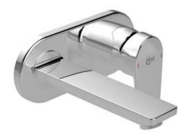
Tesi built in basin mixer kit 2, with maximum 5lt/min flow rate with 47 mm cartridge, 192 mm spout projection, hot water limiter integrated in the cartridge, cascade aerator M24x1, chrome, for combination with kit 1 A5948NU.
