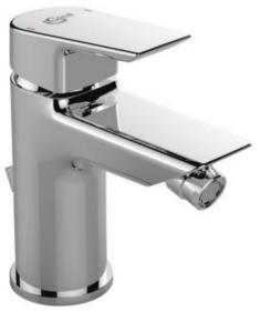
Tesi bidet mixer with 28 mm ceramic catridge, hot water limiter (separate in pack), ball joint M18x1, Easy fix, flexible hoses G3/8", pop-up rod and metal pop-up waste, chrome.
