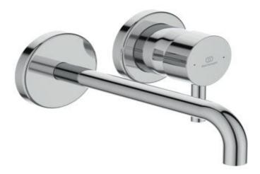
Ceraline built-in basin mixer kit 2, with 47 mm ceramic cartridge, hot water limiter, cylindrical spout, 204 mm spout projection, 2 round escutcheons, chrome for combination with A5948NU.
