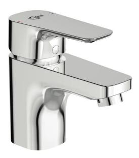
Ceraplan III basin mixer with 40 mm Click cartridge, flow rate and hot water limiter, flexible hoses G3/8", Easy-fix, cascade aerator M24x1, centering & sealing ring, pop-up rod and metal pop-up waste, chrome
