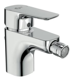
Ceraplan III bidet mixer with 40 mm Click cartridge, flow rate and hot water limiter, flexible hoses G3/8", Easy-fix, ball-joint M18x1, centering & sealing ring, pop-up rod and metal pop-up waste, chrome
