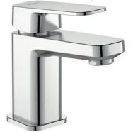
Tonic II piccolo basin mixer with maximum 5lt/min flow-rate, 28 mm cartridge, hot water limiter, flexible hoses G3/8", Easy-fix, adjustable cascade aerator M24x1, metal handle, pop-up rod and metal pop-up waste, noise class 1, chrome
