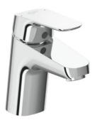
Ceraflex basin mixer with maximum 5lt/min flow rate, 40 mm ceramic cartridge, hot water limiter, Easy - fix, flexible hoses G3/8" aerator M24x1, metal pop - up waste, pop-up rod, chrome.
