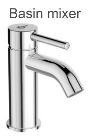
Ceraline basin mixer with maximum 5lt/min flow rate, 35 mm ceramic disc cartridge, hot water limiter, flexible hoses G3/8", Easy-fix, cache aerator M21,5x1, metal pop-up waste, pop-up rod, chrome.
