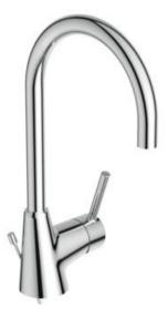
Ceraline basin mixer with high tubular spout, with a maximum 5lt/min flow rate, 35 mm ceramic disc cartridge, hot water limiter, flexible hoses G3/8", Easy-fix, metal pop-up waste, pop-up rod, chrome.
