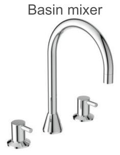
Ceraline rim-mounted basin mixer, 3 holes, with a maximum 5lt/min flow rate, a 160mm projection high tubular spout, ceramic valve G1/2" 90° left and right, aerator M24x1, Easy-fix, adaptor from G1/2" to G3/8" connection, chrome.
