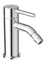
Ceraline bidet mixer, with maximum 5lt/min flow rate, 35 mm ceramic cartridge, hot water limiter, flexible hoses G3/8", Easy-fix, ball-joint aerator M18x1, metal pop-up waste, pop-up rod, chrome.
