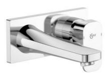
Tonic II built in basin mixer kit 2, with maximum 5lt/min flow rate, with 47 mm cartridge, 180 mm spout projection, hot water limiter integrated in the cartridge, metal handle, metal escutcheon, adjustable aerator M24x1, noise class 1, chrome for combination with kit 1 A5948NU.
