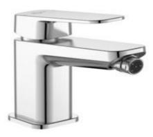
Tonic II bidet mixer with maximum 5lt/min flow rate, 35 mm cartridge, hot water limiter, flexible hoses G3/8", Easy-fix, ball-joint aerator M18x1A, noise reducer, metal handle, pop-up rod and metal pop-up waste, noise class 1, chrome.
