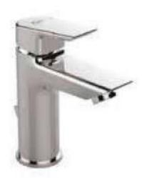
Tesi basin mixer with 28 mm ceramic cartridge, hot water limiter (separate in pack),flexible hoses G3/8", Easy-fix, cascade aerator M24x1, pop - up rod and metal pop-up waste,, chrome.
