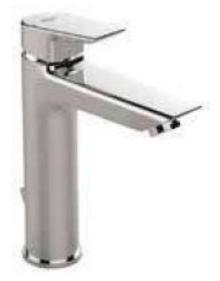
Tesi basin mixer Grande with a maximum 5lt/min flow rate, 28 mm ceramic cartridge, hot water limiter (separate in pack), flexible hoses G3/8", Easy-fix, cascade aerator M24x1, pop - up rod and metal pop-up waste, chrome.
