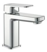
Tonic II basin mixer with maximum 5lt/min flow-rate, 28 mm cartridge, hot water limiter, flexible hoses G3/8", Easy-fix, adjustable cascade aerator M24x1, metal handle, pop-up rod and metal pop-up waste, noise class 1, chrome
