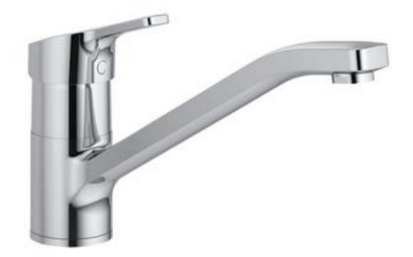
Concept 100 kitchen mixer cast spout with a maximum 5lt/min flow rate, 47mm cartridge, hot water limiter, Easy - fix, flexible hoses G3/8", chrome.
