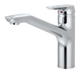
Ceramix Blue kitchen mixer cast spout with nickel and lead free waterways, 47 mm Click catridge with hot water limiter, cool body, aerator cascade M24X1, tail fixation, flexible hoses G3/8", additional foot ring, chrome.
