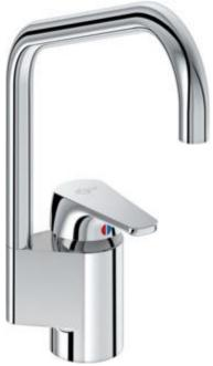
Cerasprint rim mounted kitchen mixer with 47 mm Click cartridge, high tubular spout, Easy-fix, flexible hoses PEX G3/8" and integrated aerator M16,5x1, chrome
